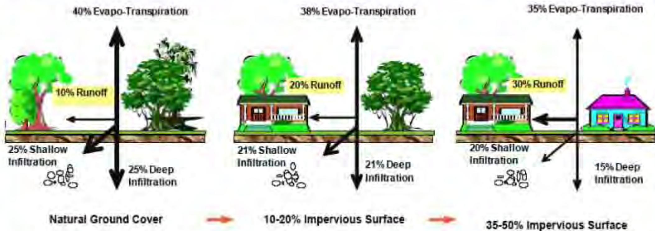
Figure 2. How impervious cover affects the water cycle.
