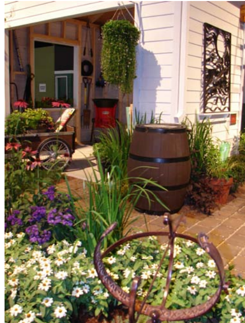
Residential rain barrels are an inexpensive and easy retrofit that reduces stormwater runoff and provides irrigation water. Photo at left: District of Columbia Water & Sewer Authority; Photo at right: Ann English.
